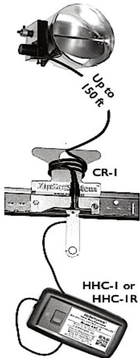
THE CR-1 bracket is the practical choice when the connection to the actuator will be in a hard ceiling and usually only a few feet from the damper. The CR-1's ingenious design allows the bracket to easily mount to any industry standard T-grid, and saves misc cost and labor time since no auxillary support framework is needed.
